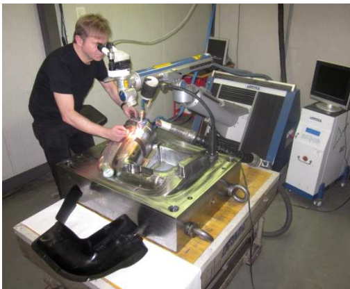
mobile repair welding
